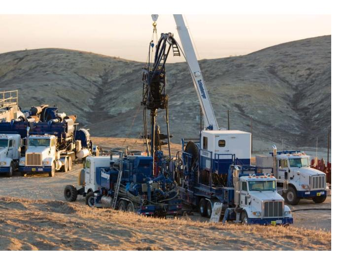
The big advantage of coiled tubing, of course, is that tripping in and out of a well is continuous. That is not only faster than making up joints of tubing, it requires fewer people on the rig floor and makes the whole operation safer.
