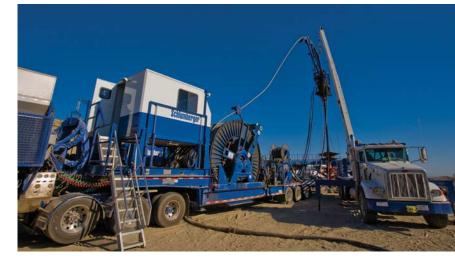
For live wells, CT perforating can run long gun strings and either drop them off or retrieve them without having to kill the well. The ability to continuously circulate through the tubing also makes it easy to spot-treat with fluids. Treating a carbonate interval with acid just before perforating, for example, creates cleaner perforations.
