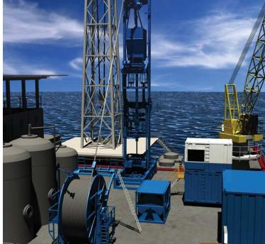
Pipe passing through the injector head straightens before it enters the wellbore. A stripper, set below the injector head, contains the packing that seals the outside diameter of the tubing and isolates pressure from the well.
