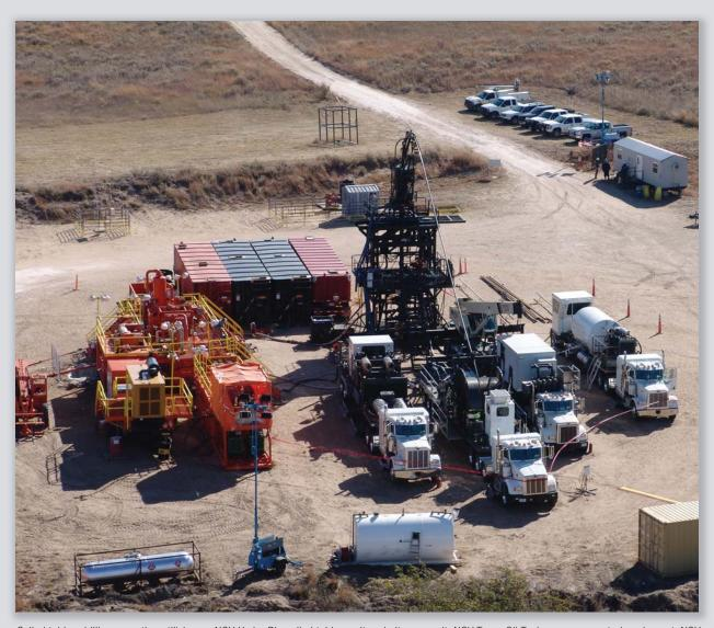
Coiled tubing drilling operation utilizing an NOV Hydra Rig coiled tubing unit and nitrogen unit, NOV Texas Oil Tools pressure control equipment, NOV CTES data acquisition system, and an NOV Rolligon twin fluid pumper.
