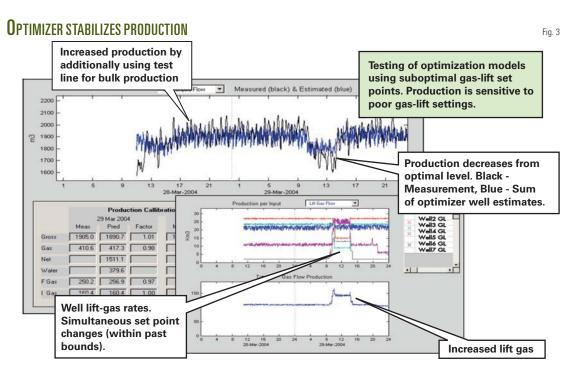
combining a well's physical models with real-time wellhead pressures and temperatures to predict three-phase flow in real time or near real time.
