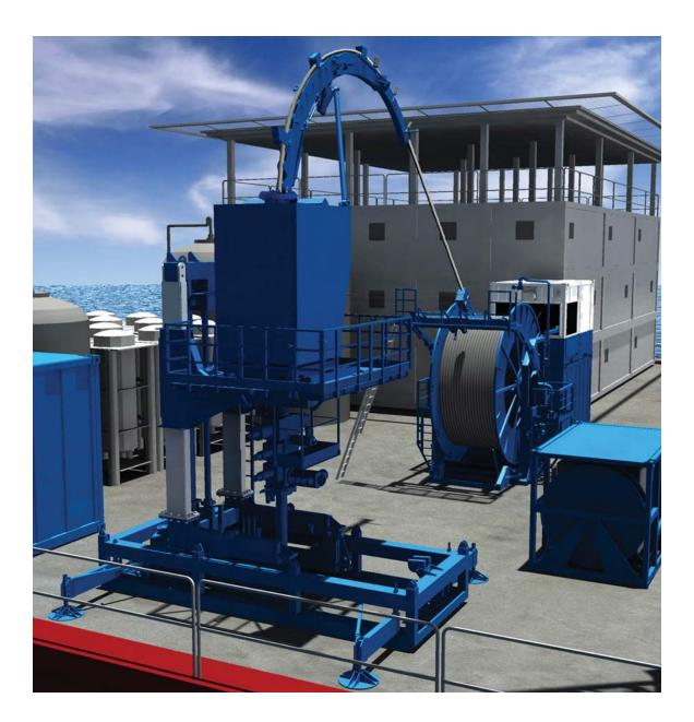
fewer offshore personnel. The design of the equipment package features fewer mechanical connections, improved control room ergonomics, and faster well-to-well cycle times. Compared to earlier systems, CT SEAS systems can also run heavier coiled tubing at increased speeds.
